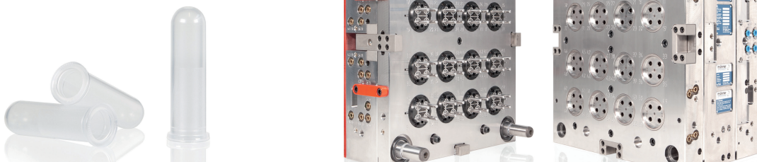
Fig. 2. A 64-cavity tool for 2-ml reaction vessels made of polystyrene with separate closure. The multipoint nozzles used can be installed to save space © Männer
