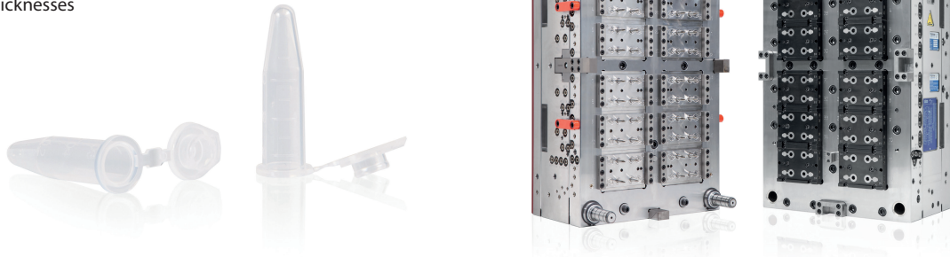
Fig. 1. A 48-cavity mold for polystyrene reaction vessels with safe-lock lids. Challenges in the process include closure with defined lid-opening force, vapor tightness, and homogeneous wall thicknesses
